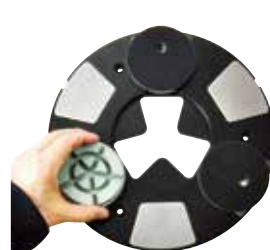
3. Attachment of resin diamonds
